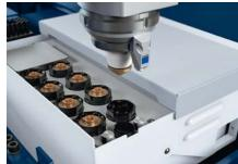
The automatic nozzle changer means that you no longer have to switch cutting nozzles by hand. The machine does it for you in just a fraction of the time.
