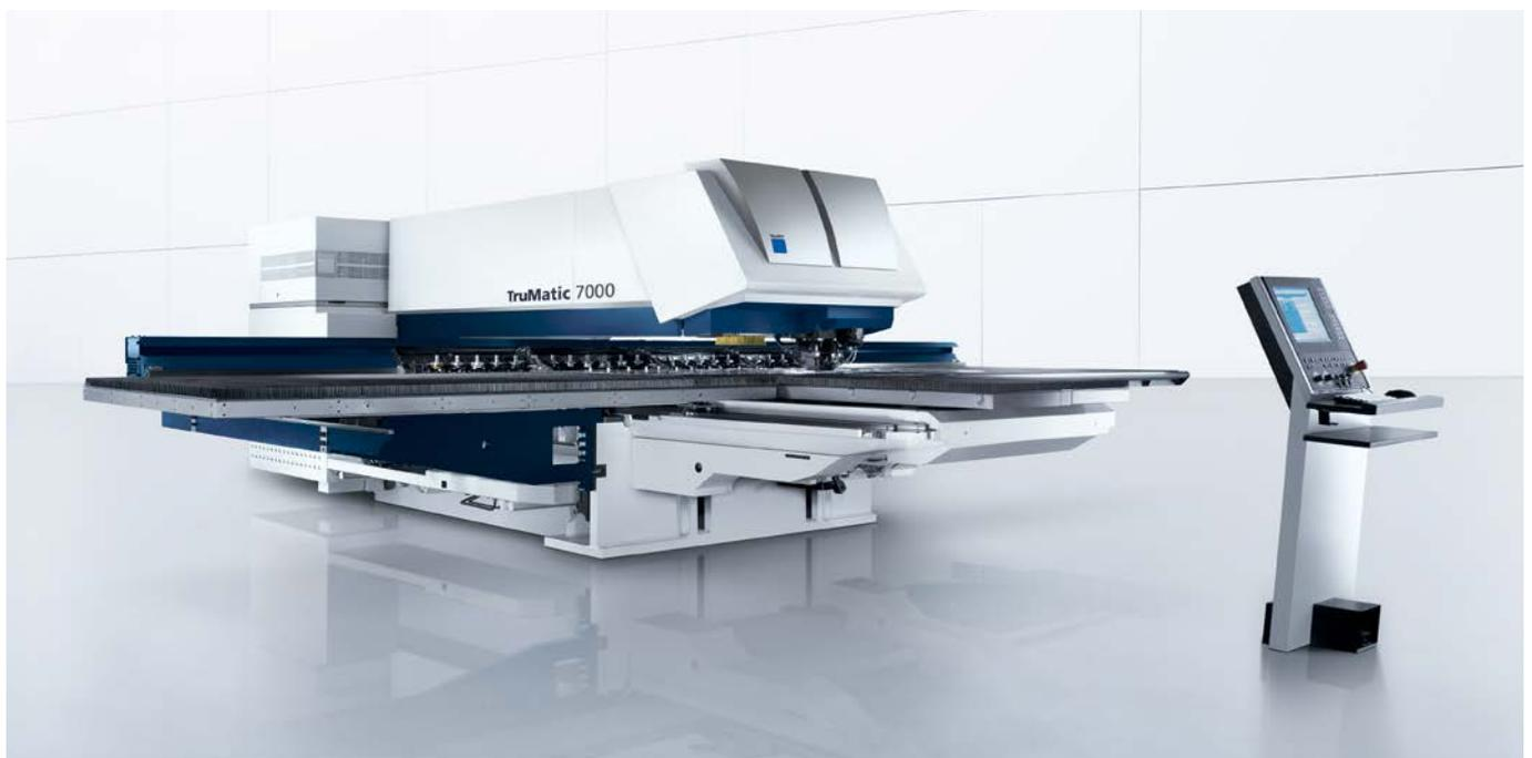
All TruMatic machines are manufactured in an open C-frame design which gives you access to both the machine and the workpiece from three sides. With this configuration there is plenty of room for both manual and automated loading and unloading. Our machines are extraordinarily stable, ensuring high levels of accuracy and a long service life.
