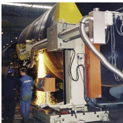
Back gouging of weld seams
