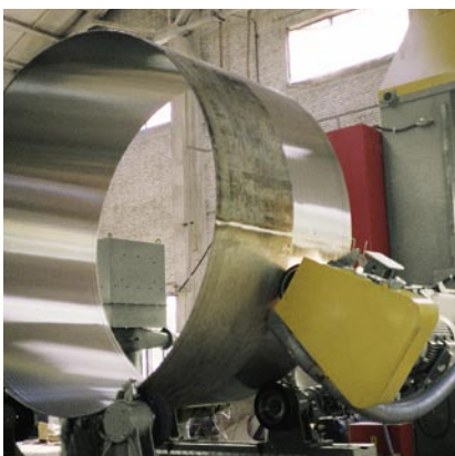
Surface grinding internal and external on vessels
