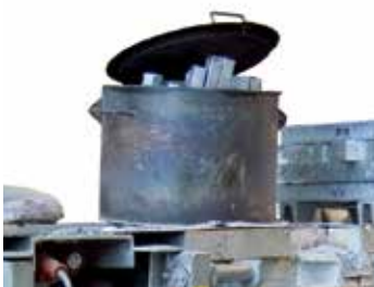
Charging funnel for ingots
