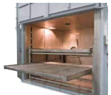
Pull-out drawers for heavy loads
