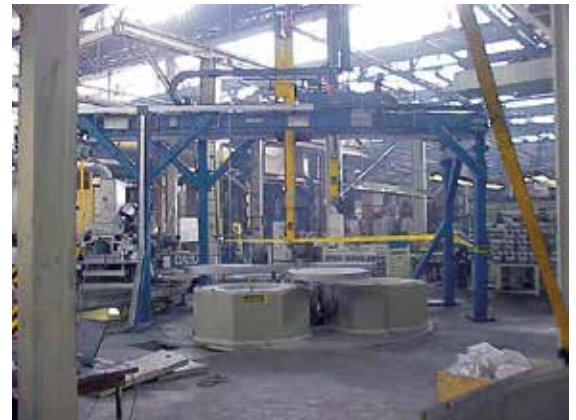
Rotary table system with 3 x T 150/11
