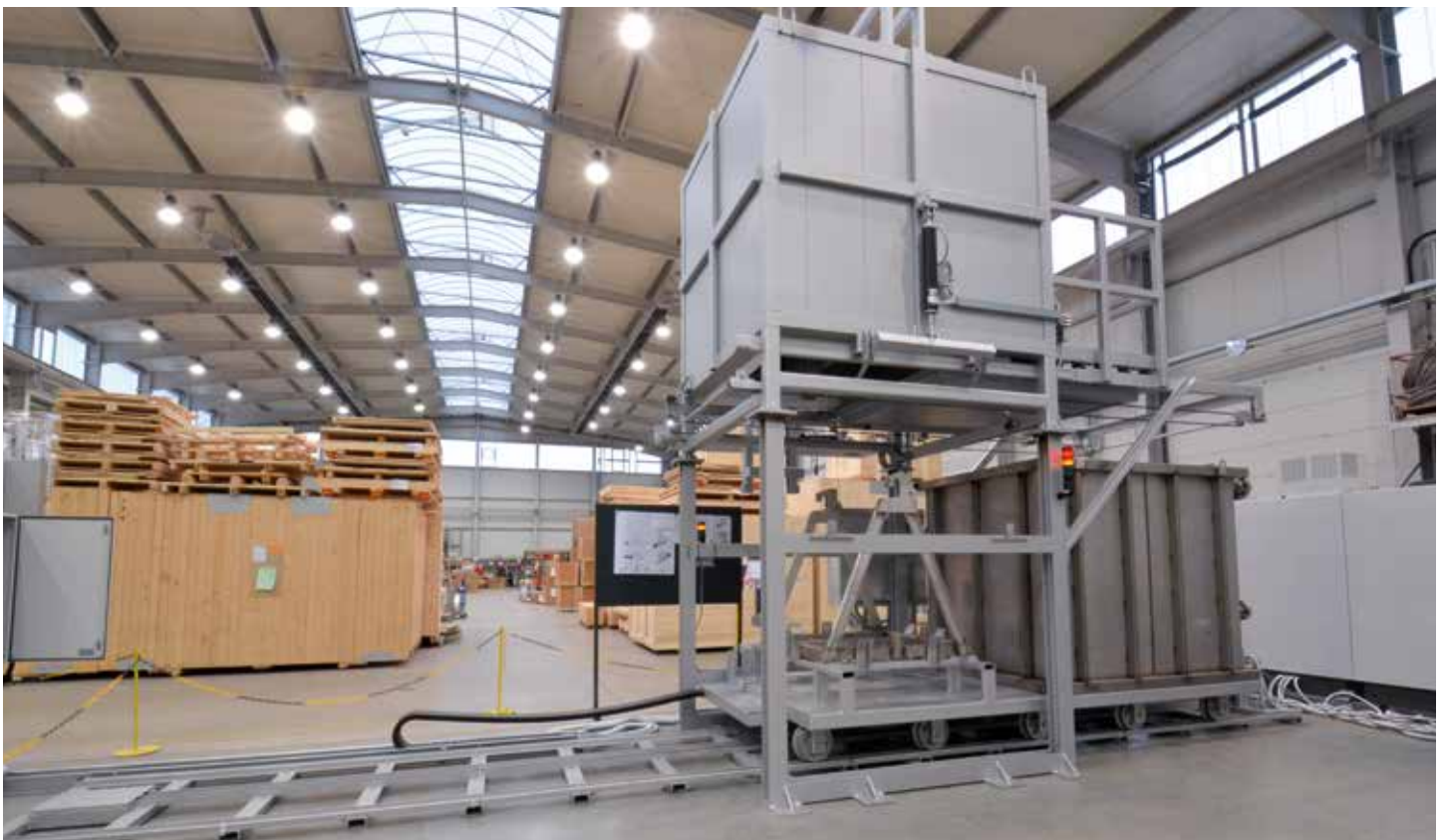
Quench and temper system with drop-bottom furnace FS 2200/60AS and quench bath
