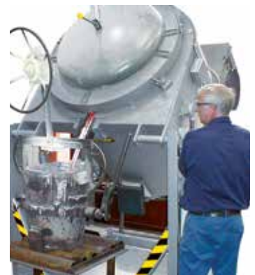
KB 240/12 for melting aluminum alloys
