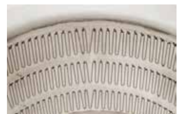
Meander heating elements
