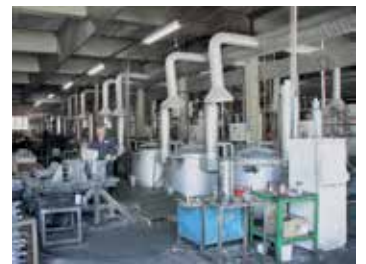
Recuperator burner for aluminum melting furnace 16 x TBR 110/12 and 2 x TBR 180/12
