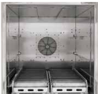
Roller conveyor in furnace N 250/85HA
