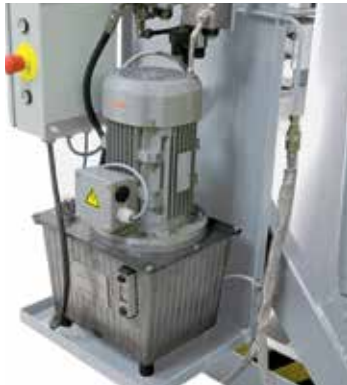
Hydraulic system with flame resistant hydraulic fluid
