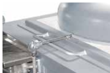
Bath control with thermocouple in the melt
