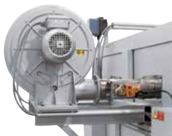
Cooling fan for accelerated cooling
