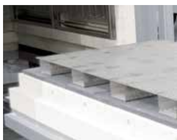
Charge support in an air circulation bogie hearth furnace for 850 °C
