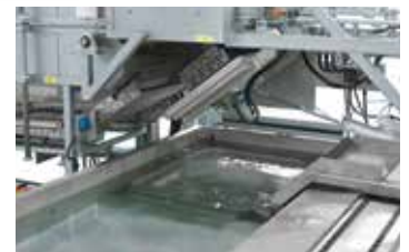
Drop bottom for quenching within 5 seconds
