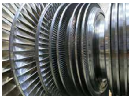
Turbine rotor shaft
