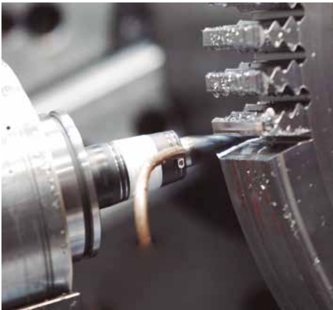
Finishing of turbine Blade fir tree roots
