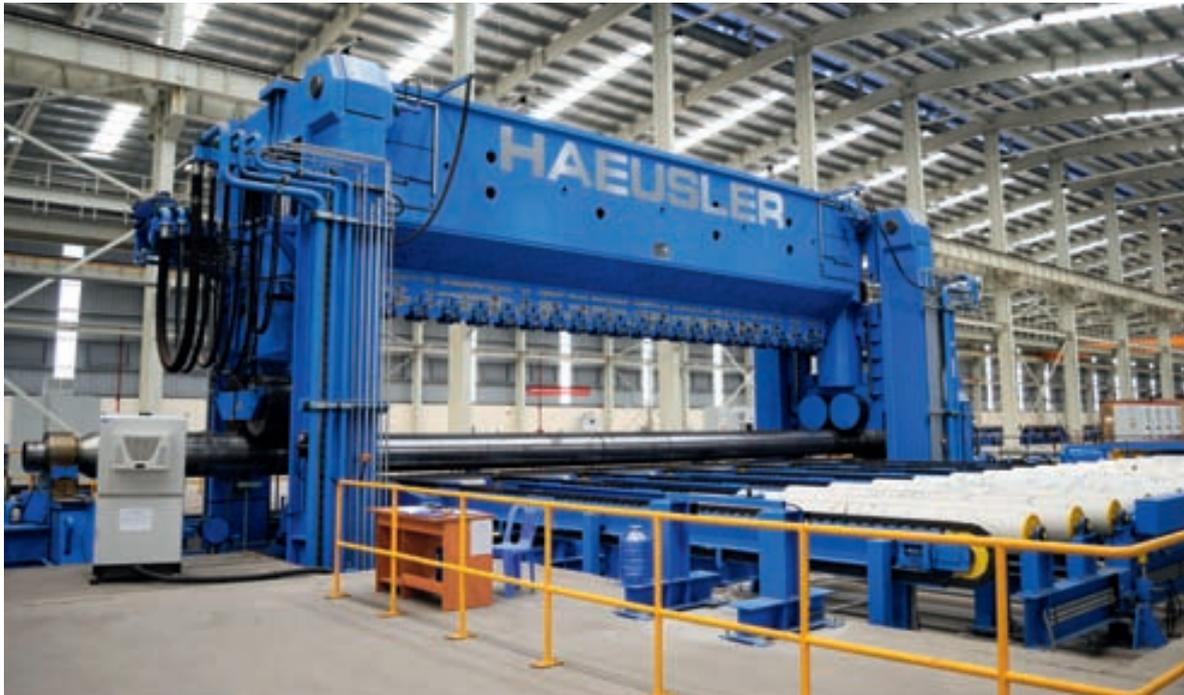
The first RB LSAW pipe mills were already clearly superior to other forming processes such as JCO and UOE in regard of out-of-roundness tolerance and productivity, especially when taking into consideration the differences in initial cost. However the maximum pipe wall thicknesses were limited.
